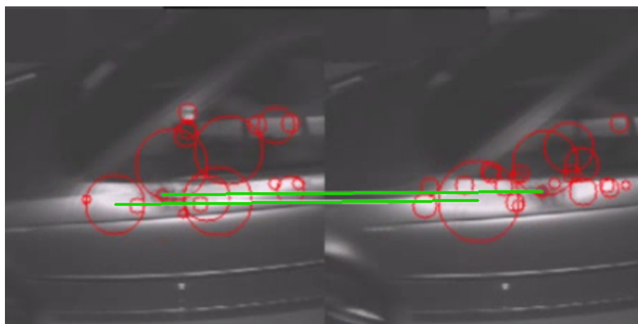
Figure 6.20: SURF extraction of moving car. Features are mainly found in oversaturated areas or reflections. [HLK13b]
