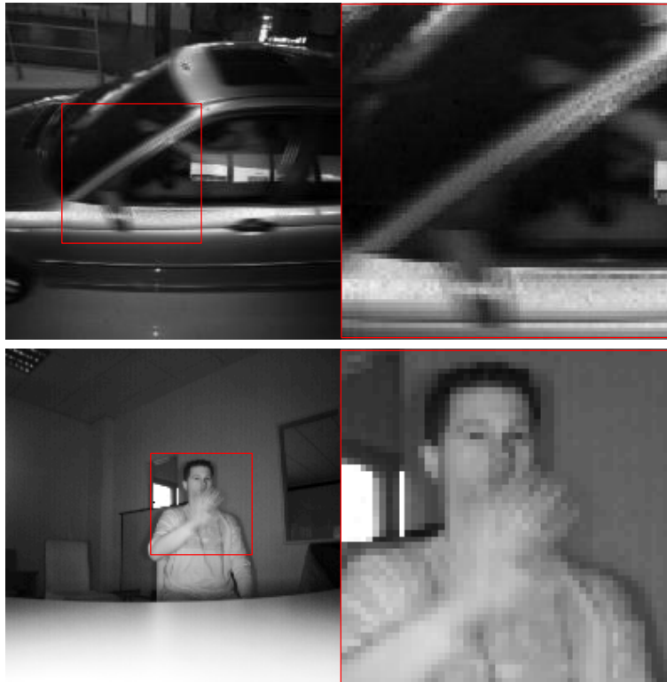
Figure 4.2: Top: demodulation of the car's phase image sequence and a corresponding closeup. Bottom: a moving hand scene and a corresponding closeup. Left: motion areas are marked red. Right: The closeups of the marked motion areas.[HLK13a]
