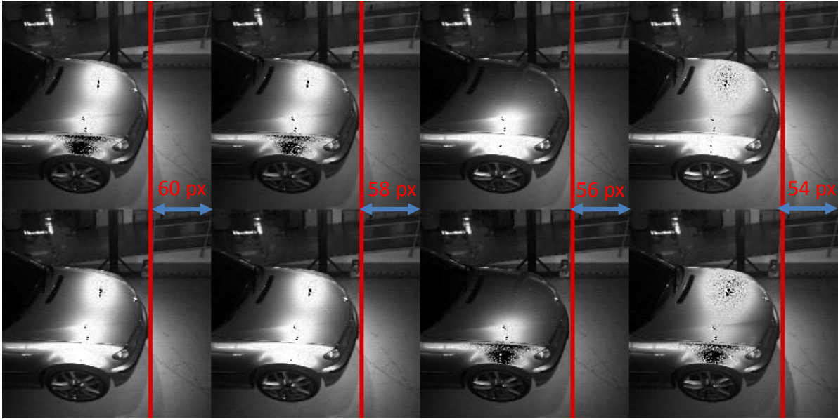
Figure 6.5: The four phase images with marked movements of the car (about 6 pixels between phase 1 and 4). Top: phase channels P_{A1} - P_{A4} . Bottom: phase channels P_{B1} - P_{B4} . [HLK13b]
