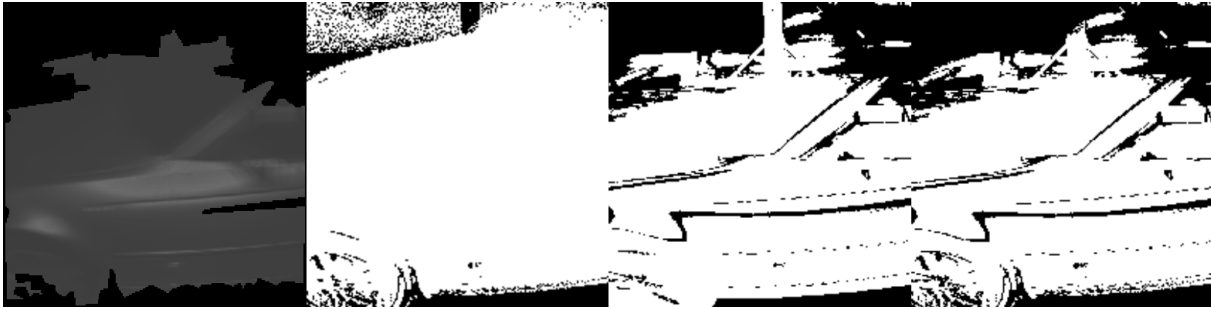
Figure 6.11: Left to right: segmented background image after applying the final morphological closing; distance segmentation; intensity segmentation; combination of distance and intensity segmentation. [HLK13b]
