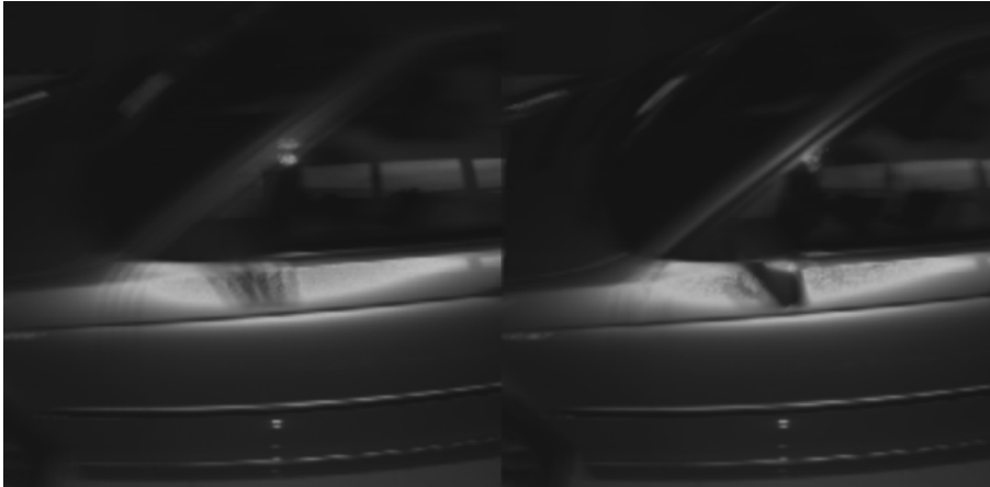
Figure 6.6: Left: motion artifacts of the moving car, e.g. at the mirror (intensity image). Right: successful motion compensation. No more artifacts are visible at e.g. the mirror (intensity image). [HLK13b]
