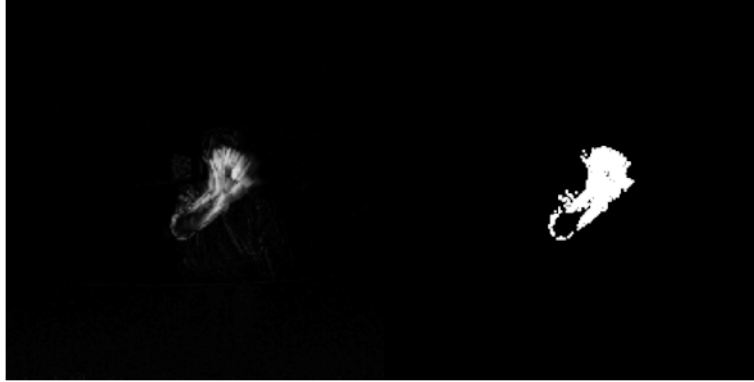
Figure 4.4: The moving hand from Fig. 4.2 with extracted motion artifacts. Left: the motion image M calculated using Equation 4.4. Right: the binarized image B thresholded using Equation 4.5. [HLK13a]
