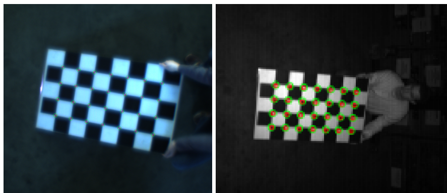
Figure 2.6: Reprojection results after applying the estimated transformation between the RGB (left image) and the PMD (right image) camera. [HLK13b]
