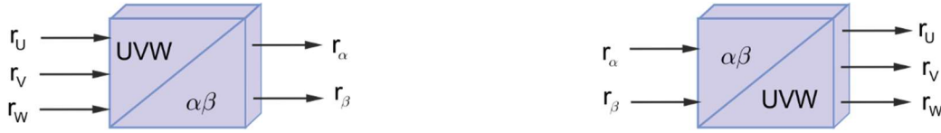
Fig 2.3. Symbol for the transformation of coordinates between the \alpha, \beta - and the UVW -coordinates
