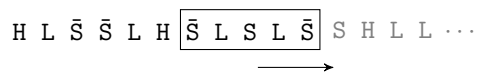
Figure 1.1: A stream of signals with a sliding window of length n = 5 . Signals in gray will arrive in the future.
