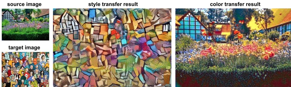
Figure 4.31: An example of style versus color transfer. Both methods use the same source and target images. The style includes both texture and color, which represents the style of the painting in the target image. The color transfer result has the target image's color palette while maintaining clear content from the source image. The style transfer result is created using Gatys et al. method [GEB16], and the color transfer result is created by using our perceptual color similarity network.
