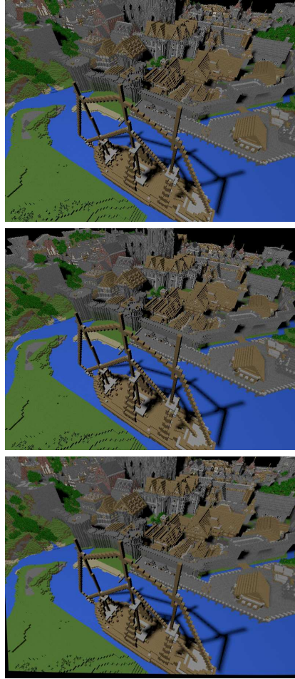
Figure 2: From top to bottom: undistorted image of size 800,600 rendered with intrinsic parameters c_x = 399.5, c_y = 299.5, f_x = f_y = 400 , distorted image rendered with parameters k_1 = -0.05, k_2 = 0.01, p_1 = 0.03, p_2 = -0.01 , and undistorted image produced from the distorted image by OpenCV using the same parameters.
