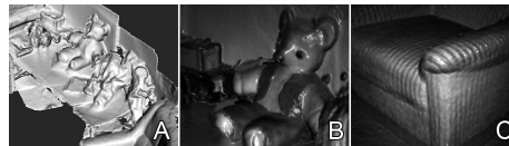
Figure 10. A: the PMD scene acquired with a PMD ToF camera. B and C: close-ups using per-pixel intensity values for coloring.
