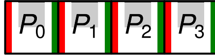
Fig. 1. Four horizontally neighboring sensor pixels in the dual-readout approach with A readout circuit (red), B readout circuit (green), and optically active area (gray).
