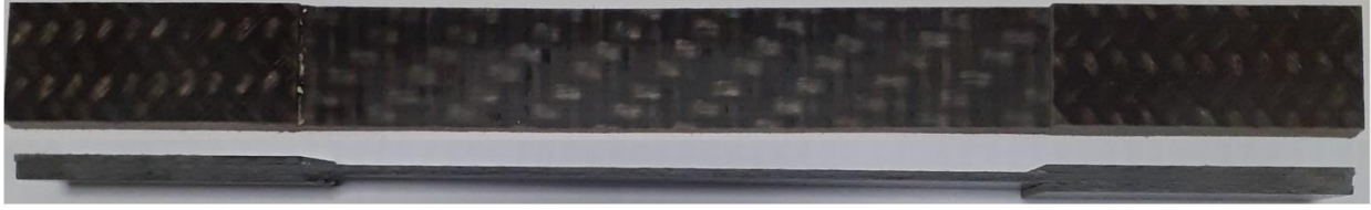
Figure 3.3 Tensile test specimen with four end tabs glued. Rovings of the glass fabric are also visible indicating the direction of material
