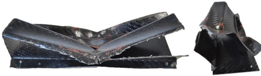
Figure 6.17 Photos of drop tower three point bending of hat profile during the test at different deformations along negative z-axis. The deformed geometry of profile after the test is also shown
