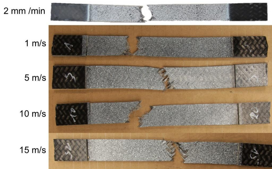
Figure 6.6 Tensile shear specimens tested at different speeds. More specimen photos are given in Annex 12.2.10
