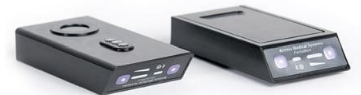
Abbildung 20: PortaMon -NIRS-Sensoren (Artinis Medical Systems B.V., 2015)
