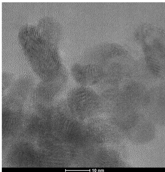
Figure 4.10: TEM images of highly crystalline \text{LaF}_3:\text{Ce}^{3+}\text{Tb}^{3+} NPs prepared in 1:1 ratio of EG:PVP and dispersed in a suspension of Milli-Q water and 25 mmol PVP.
