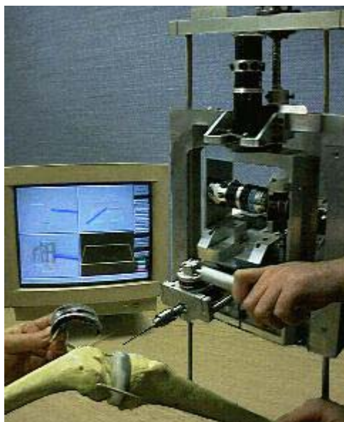
Figure 3.7. ACROBOT, special purpose Hands-On robot for knee surgery
