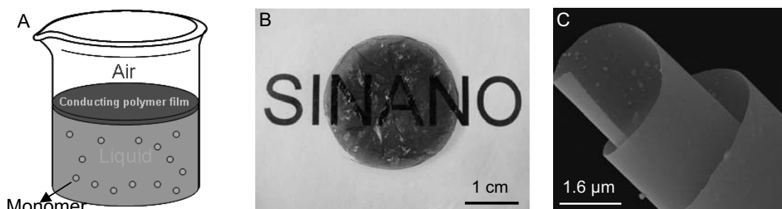
Figure. A) The schematic of free-standing conducting polymer film growing at air/liquid interface. B) The digital image of the film floating on water surface. C) The cross-section SEM image of the film.
