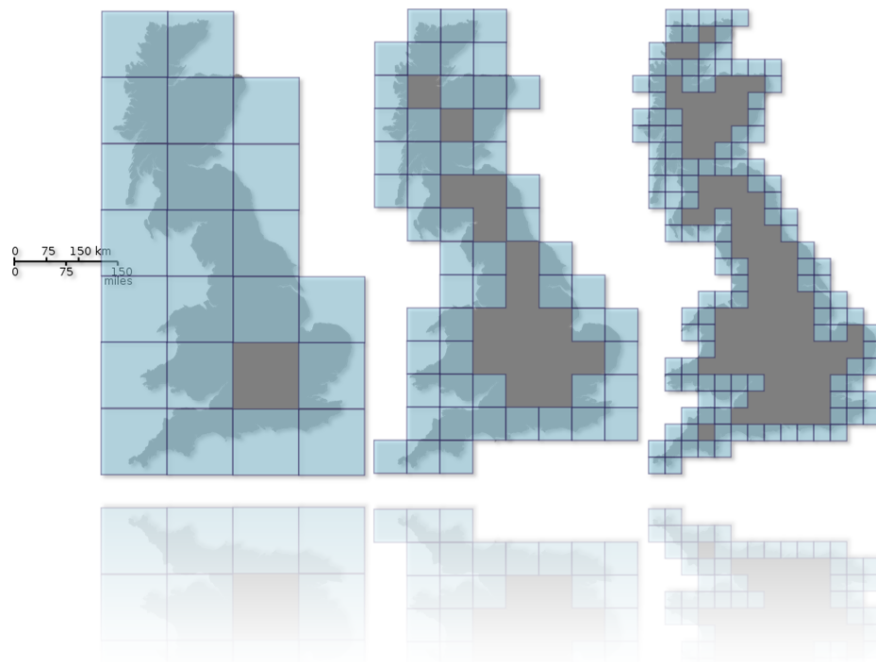
Figure A.3: Estimating the box-counting dimension of the coast of Great Britain
