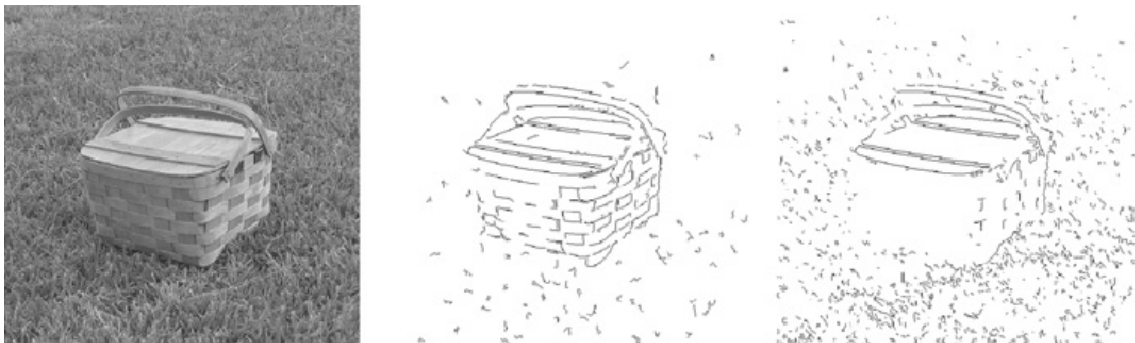
Figure B.9: Simulated surround suppression model by [344] (Middle) of an input image (left), compare to the plain results of the Canny edge detector (right). Picture modified from [344]
