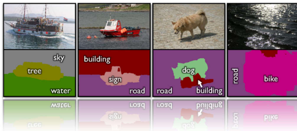
Figure 11.2: Examples where recognition works less well. Input test images with corresponding color-coded output object-class maps. Even when recognition fails, segmentation may still be quite accurate. Picture taken from [433]
