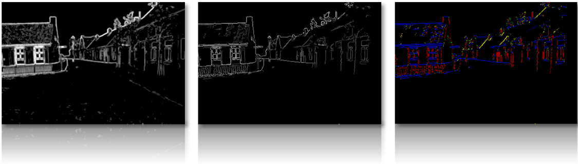
Figure 11.7: Gabor Voting. Left: Edge gradients intensity coded from 0 to 1. Middle: Gabor voted image after non-maximum suppression. Right: Edge orientations color coded \approx 0^\circ (blue), \approx 90^\circ \vee -90^\circ (red), \approx 45^\circ (yellow) and \approx -45^\circ (green)
