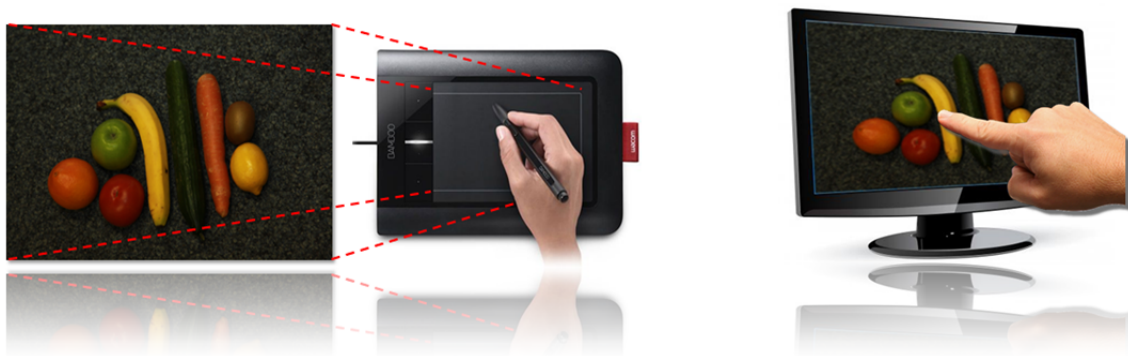
Figure 5.2: Left: Pen to tablet interface with absolute coordinates, Right: Touch screen working directly on the acquired image
