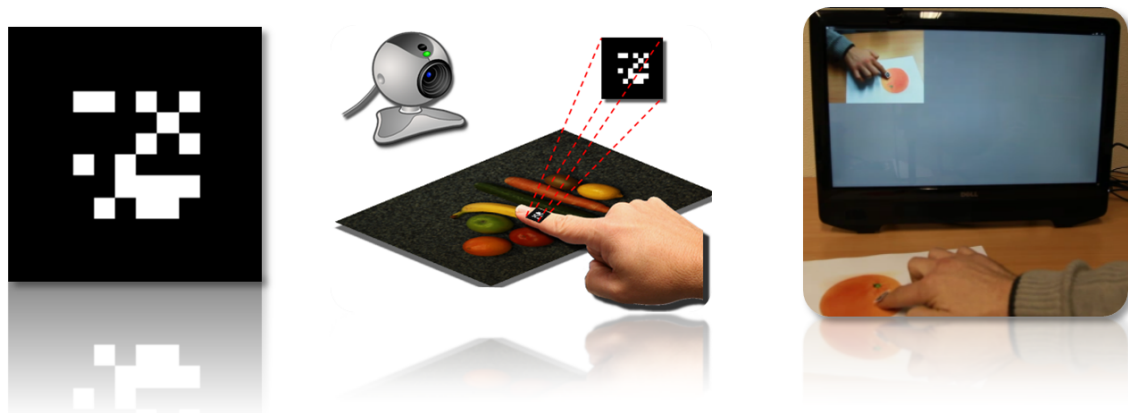
Figure 5.3: Left: A typical “marker” to be tracked. Middle: Finger position (x, y) is tracked using a marker system and estimated within the image. Right: The system in process
