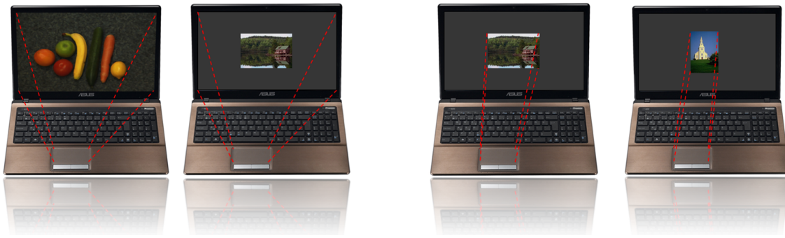
Figure 5.4: A common notebook’s touch pad switched to absolute coordinates. Left: Image rendered in the center of the touch pad. Right: touch pad mapped to the region of the image
