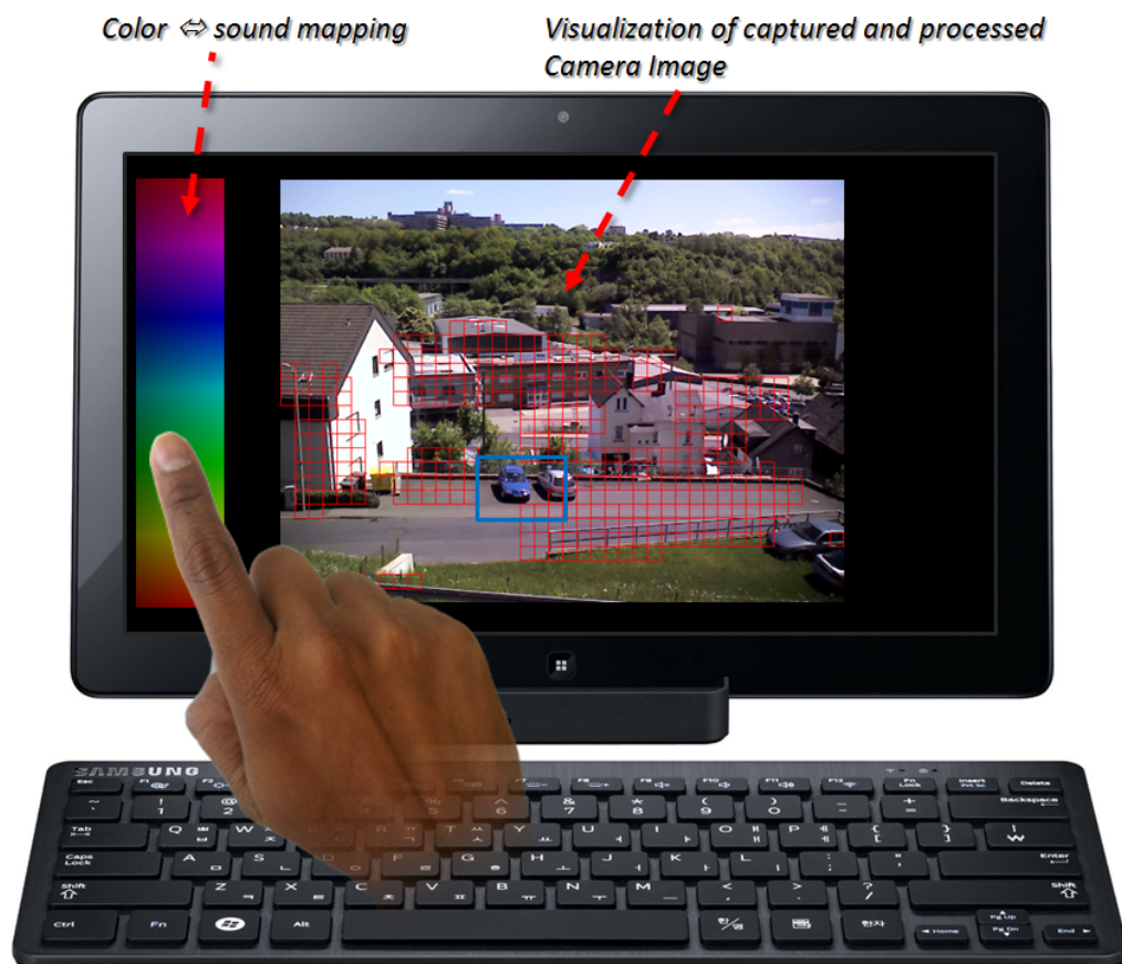
Figure 14.2: Illustration of a captured and pre-processed image on the Samsung Slate 7 tablet Pc. The color to sound mapping is visualized in the left part of the screen
