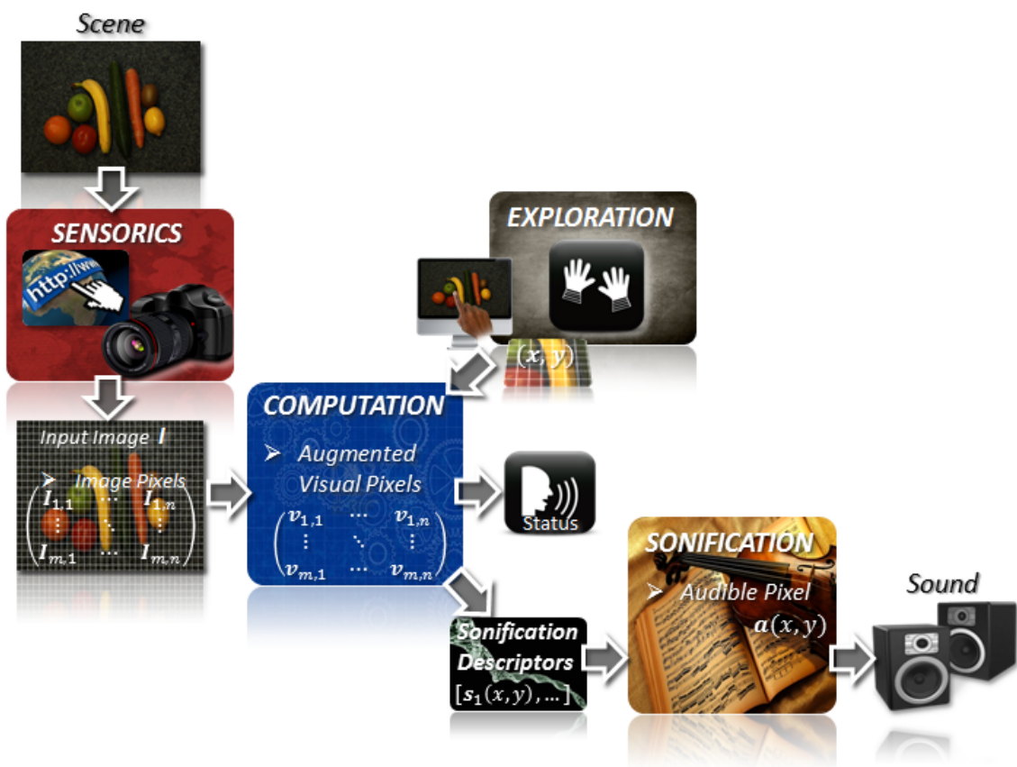
Figure 4.1: The Modular Computer Vision Sonification Model
