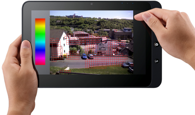
Figure 1: The Explorative Image Sonifyer System on a regular Microsoft Windows 7/8 tablet PC. Detected man made structures are highlighted (using squares). On the left side, the color to sound mapping
