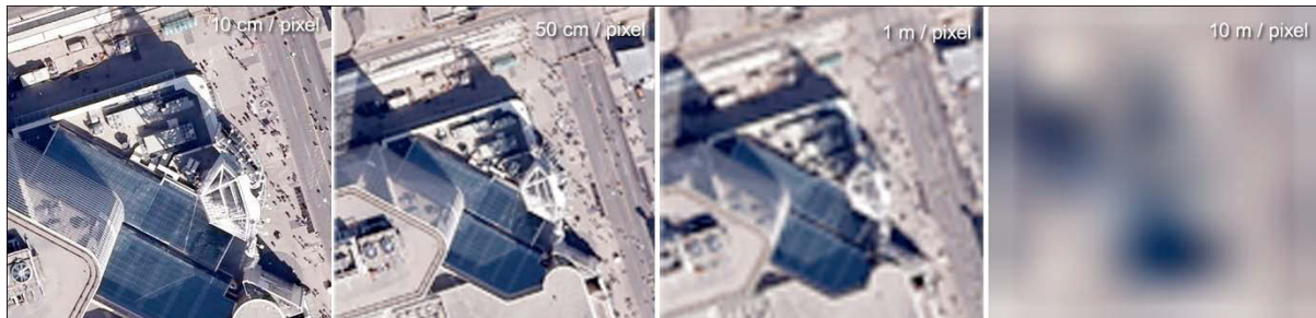
Figure 2.4 - aerial photograph at various spatial resolutions: 10 cm / pixel, 50 cm / pixel, 1 m / pixel, 10 m / pixel.
