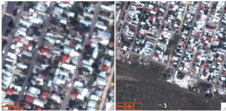
Figure 6.3 – Grid cells size: (a) optimal, (b) suboptimal (a) the patch contains solely the concept class of interest (b) the patch contains information about other classes
