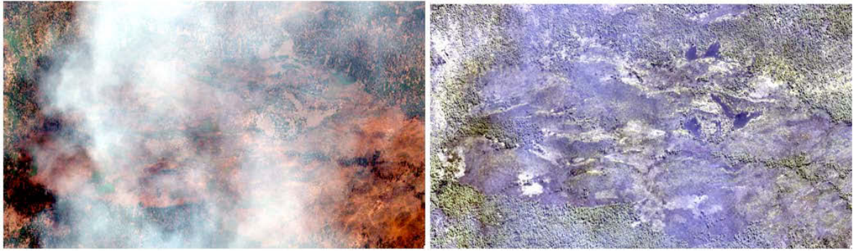
Figure 6.39 -WorldView-2, Forest areas – note how the algorithm allows visualization under plumes, Natural Color (bands 5,3,2) & New Visualization (bands 8,7,6)
