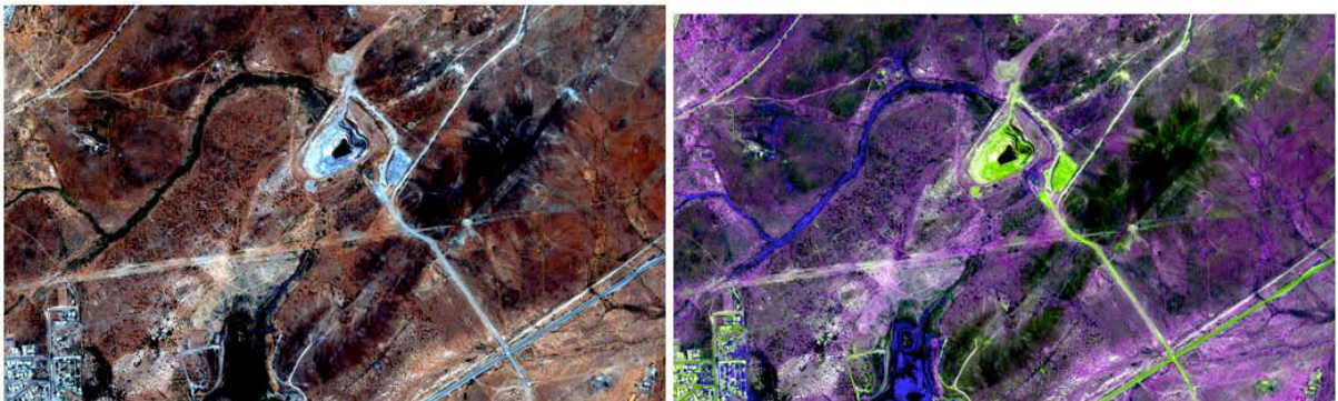
Figure 6.41 - WorldView-2, Man-made objects in the desert Natural Color (bands 5,3,2) & New Visualization (bands 4,1,7)
