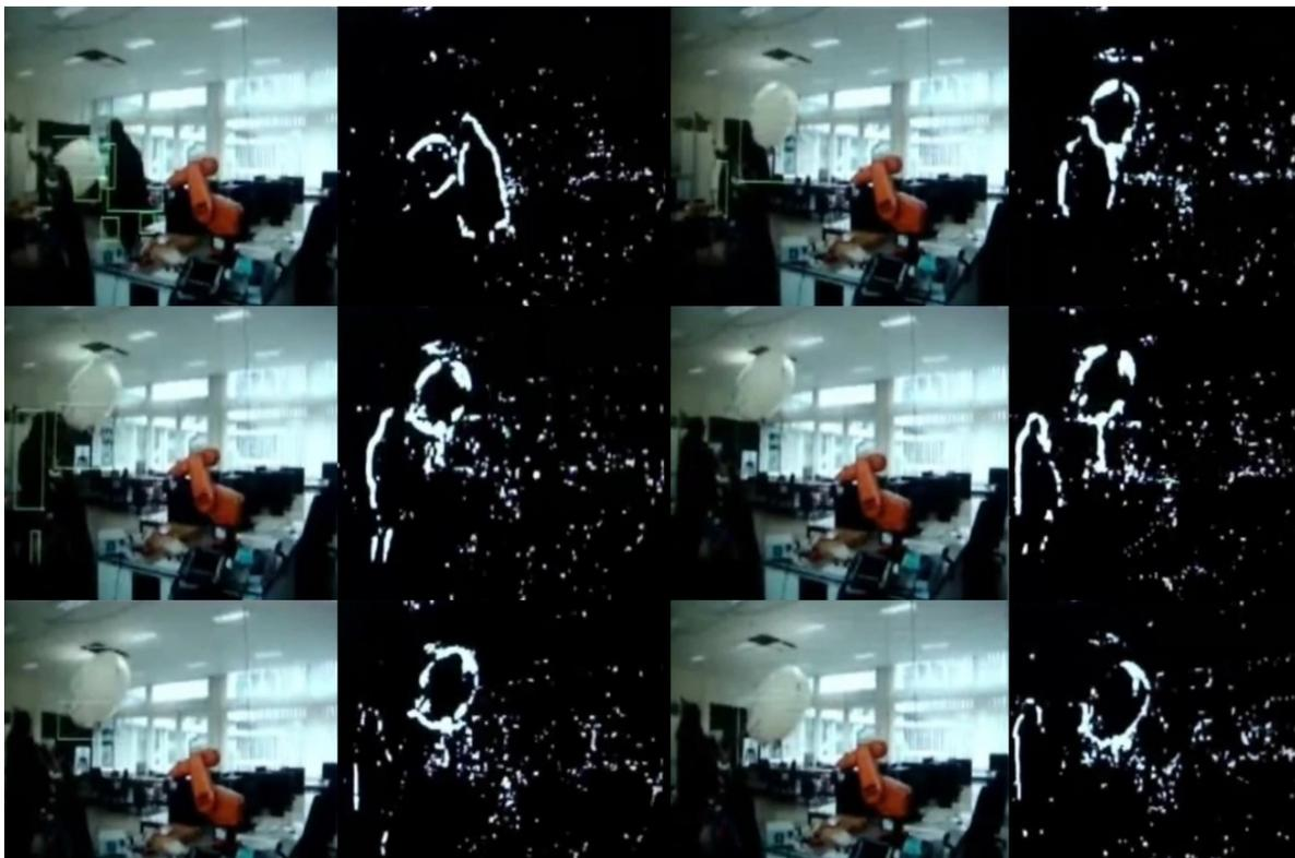
Figure 4. 1a The optical flow sequence of images to detect blimp robot.
