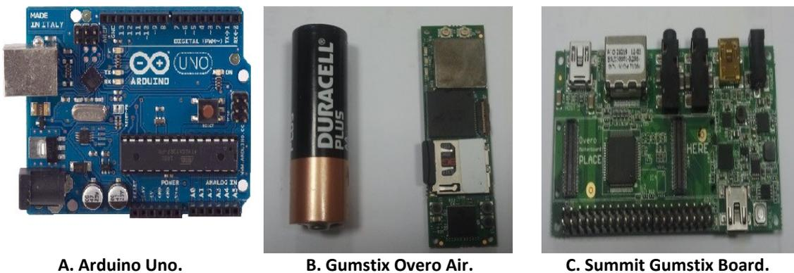
Figure 3.7 The core of the blimp system.
