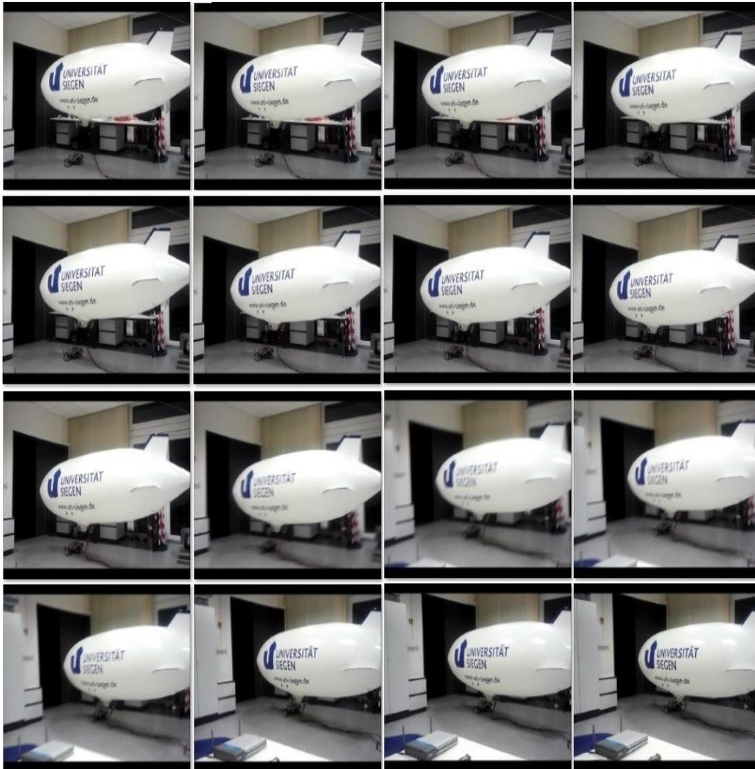
Figure 5. 30 Blimp robot lands on the ground robot.
