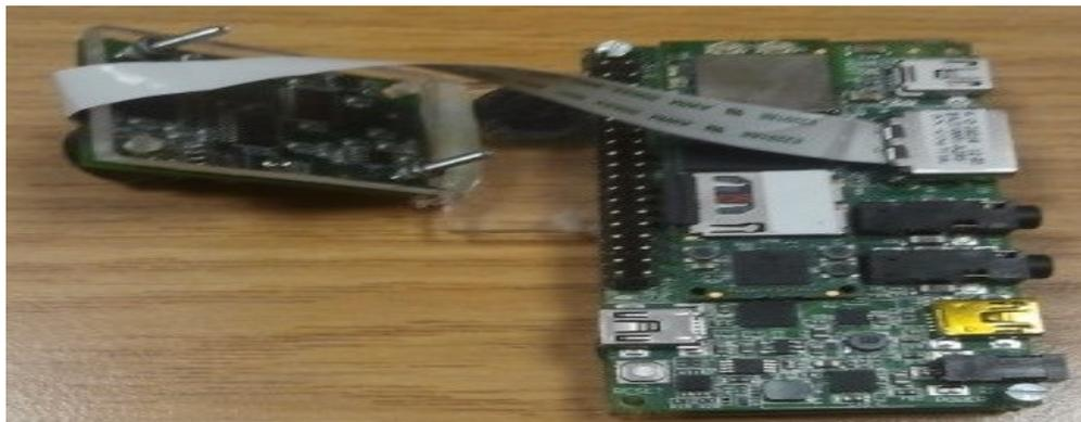
Figure A-A2 Caspa camera mounted to Gumstix Overo Air.
